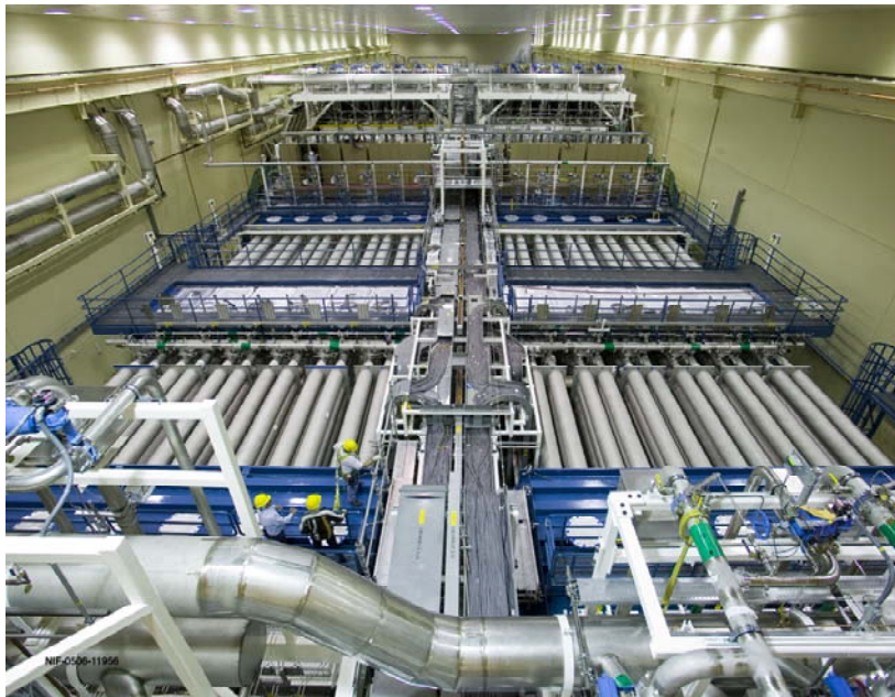
View of 1 of 2 laser bays 192 laser beams; 1.8MJ; 500TW
