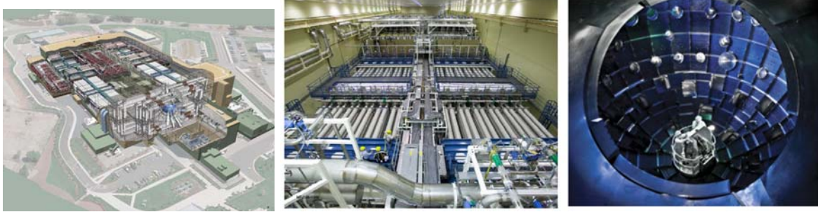
Fig. 1.13 NIF 1.8MJ laser system (left) and photographs of the laser bay and target chamber (right)
