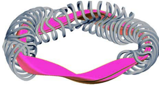
Fig 1.11 Stellarator magnetic field coils and plasma
